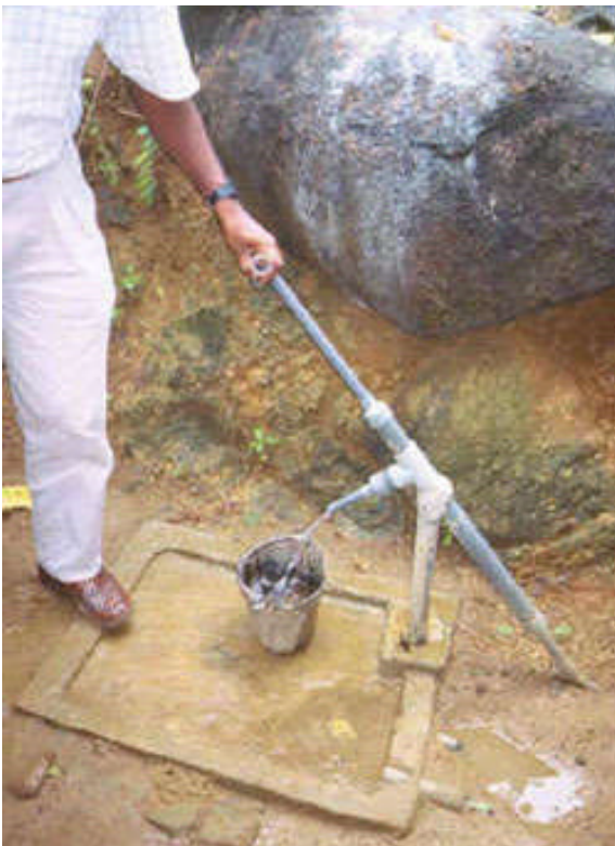
Figure 17: The Tamana pump installed at Batalahena
